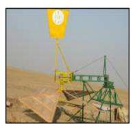
• During Jan 2010 to March 2011, fifth model was developed with supporting structure for turbine blade was added, furling tail mechanism and modification in crank mechanism
