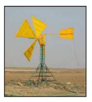
• In Feb 2009, forth model a tilting mechanism facility was provided to tilt and lower down the wind mill easily through wire rope at a safe position
