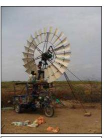
During the dry span of the rainy season, we did the trials to measure the performance of the power generating windmill. Ammeter, voltmeter, 24 volt battery and anemometer are the instrument used to collect readings.
